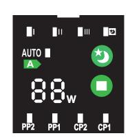
Operating functions - control buttons. NCE PS circulator could work: with curves at proportional pressure with curves at constant pressure with curves at fixed speed
